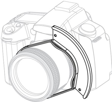
Note: The holes at the ends of the marker board are for alignment during manufacturing. They will not be used when setting up the marker board.
