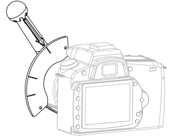
2. When using the hard stops, attach them onto the top edge of the marker board, at the focus stop positions. Position the marker board such that only the FocusShifter arrow comes into contact with the hard stop.
