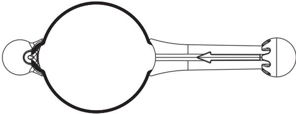
3. Position the Balance at the opposite end of the belt from the FocusShifter handle, and place the assembly on the lens.
