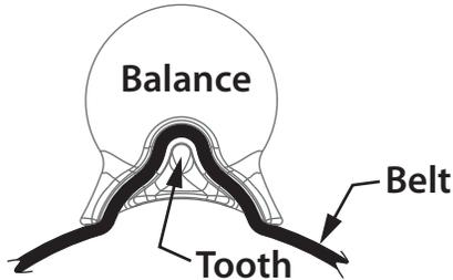
2. The belt is fully inserted when it slides behind the tooth and becomes captured in the slot.
